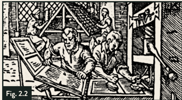
Fig. 2.2 “One printer is shown removing a newly printed sheet from the press while the other one inks the type” (Meggs 78).
